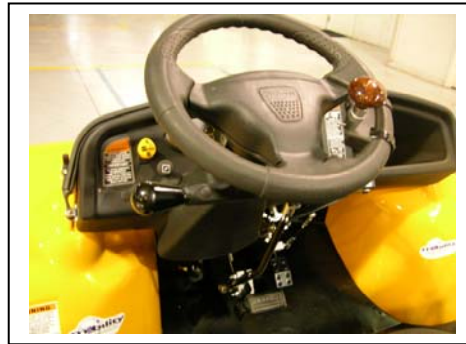
CUB CADET Hand Control Installation Photos
