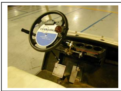
GOLF CAR Hand Control Installation Photos
