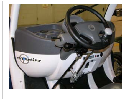
GEMCAR Hand Control Installation Photos
